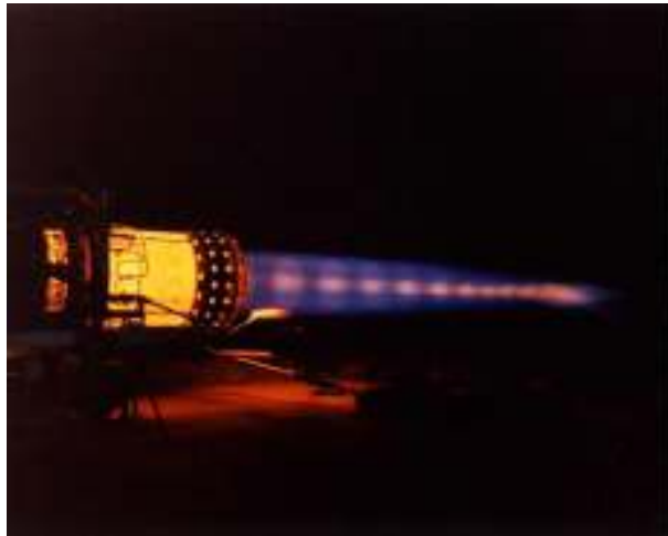
(Note blue colored cone/flame and shock diamonds in J-58 exhaust)
